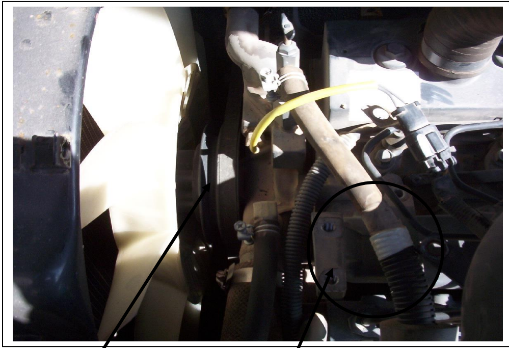
Open pulley for compressor
